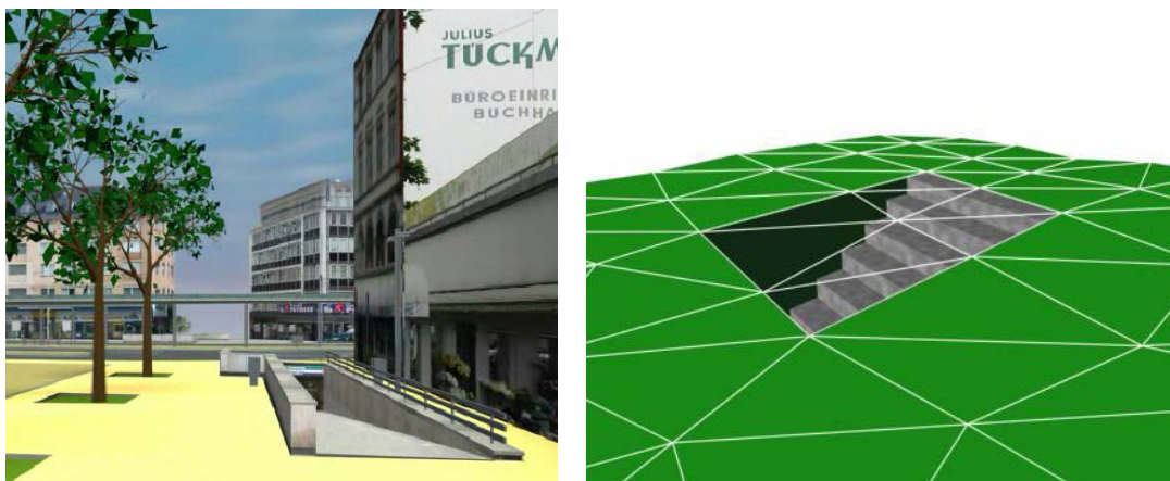
Fig. 4: Closure surfaces to seal open structures. Passages are subsurface objects (left). The entrance is sealed by a virtual ClosureSurface , which is both part of the DTM and the subsurface object (right) (graphic: IGG Uni Bonn).
